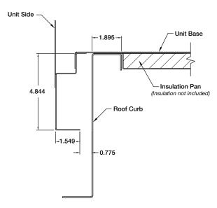
**Curb Cap Details for Factory Supplied Roof Curbs**
